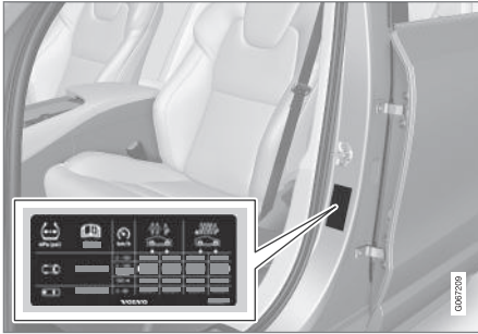
Location of the tire pressure placard
