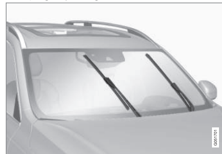
Windshield wipers in the service position.
