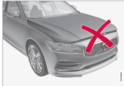
Hood not completely closed.
