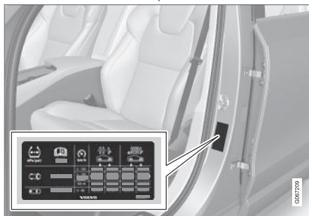
Tyre pressure label location
