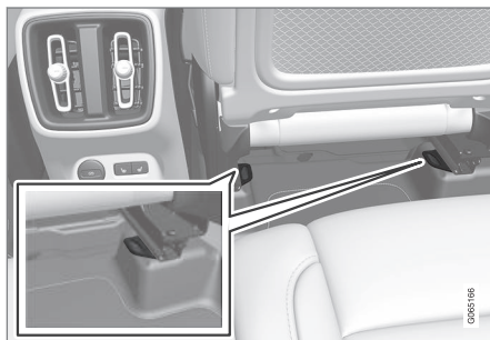
Mounting point locations in the rear seat.
