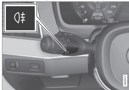
Button for rear fog lamp.
