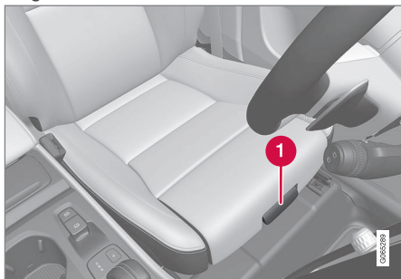
Control for seat cushion adjustment.
