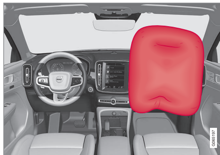
Passenger side front airbag.
