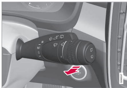
Washing function, right-hand stalk switch.
