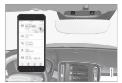
For example, you can lock and unlock the car or check the fuel level directly on a phone via the Volvo On Call app. If an accident occurs, emergency assistance can be sent to the car in the form of e.g. ambulance and police. Roadside assistance can be called for less urgent problems, such as a puncture.
