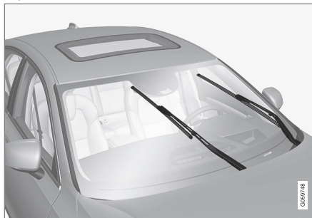
Wiper blades in service position.
