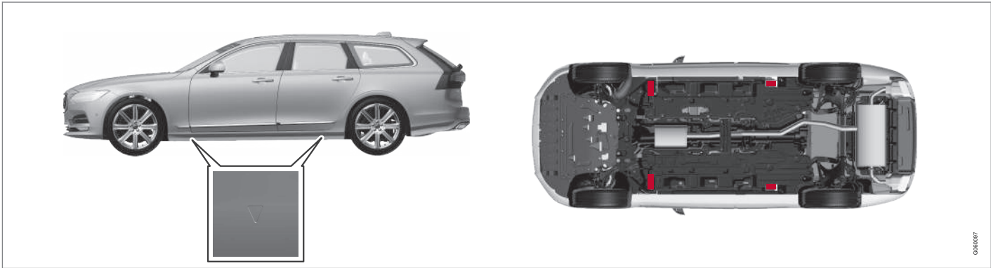
The triangles in the plastic cover indicate the locations of the lifting points (marked in red).
