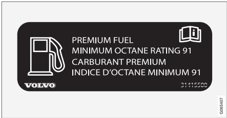
Illustration 2: Decal on the inside of the fuel filler flap on vehicles that require premium fuel 17 .
