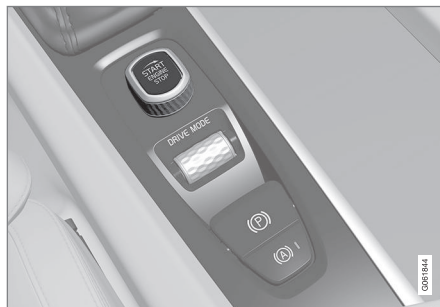
Start knob in the tunnel console.
