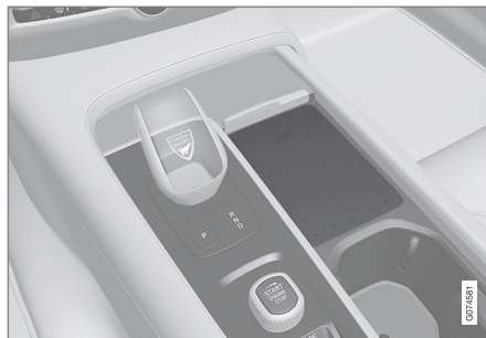
Wireless phone charger in the tunnel console.
