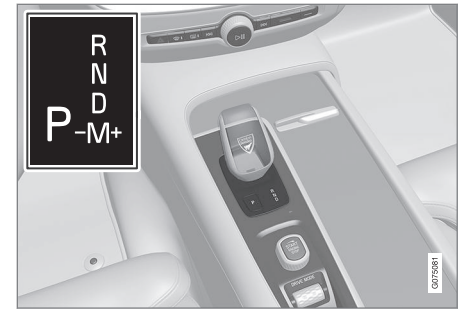
Overview of small gear selector and gear shift pattern in the instrument panel.
