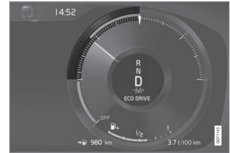
Eco gauge in 12" instrument panel*.
