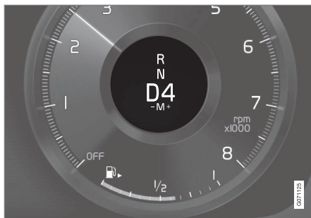
Instrument panel when shifting gears using steering wheel paddles, small gear selector.
