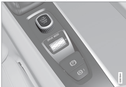
Start knob in the tunnel console.
