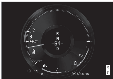
The driver display indicates charging during electric motor braking.
