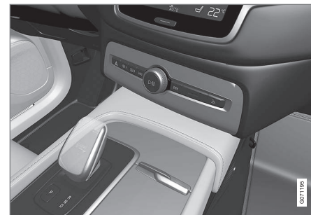
Overview of the small gear lever where it is not possible to deactivate the gear selector inhibitor.
