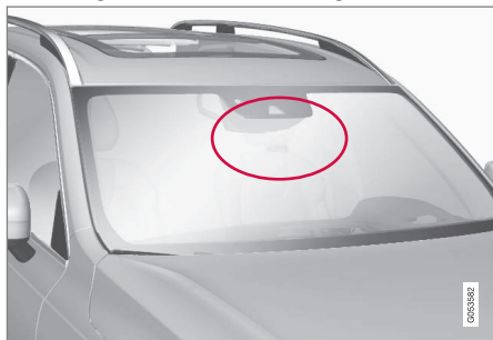
Location of the camera unit
