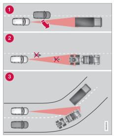
The radar sensor's field of vision
