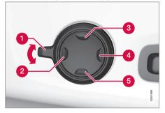
Activate the multifunction control by turning the control **1** upward/downward. The seat settings view will appear in the center display.
