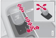
Gear selector and gear selector positions overview.
