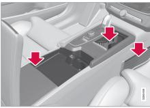
Storage compartments with cup holders, electrical outlets, net pocket\* and USB ports in the tunnel console.
