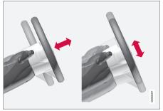
The steering wheel's reach and height can be adjusted.
