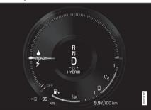
The hybrid gauge shows the ratio between the electric motor's current power consumption and the remaining available power. This information is shown in various ways.
