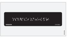
**Wehicle Identification Number (VIN).** The VIN plate is located on the top left surface of the dashboard. The Vehicle Identification Number (VIN) should always be quoted in all correspondence concerning your vehicle with the retailer and when ordering parts.
