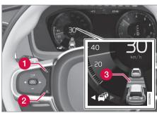
Controls for setting a time interval.
