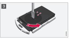
3 Use a screwdriver or similar object to turn the battery cover counterclockwise so the markers point to **OPEN**.
