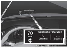
The head-up display projects warnings and information related to speed, cruise control functions, navigation, etc. onto the windshield in the driver's field of vision. Traffic information and incoming phone calls can also be shown on the head-up display.
