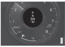
Instrument panel when the paddles are activated for shifting.
