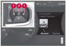
Examples of messages in the instrument panel and the right-side steering wheel keypad. The illustration is generic - details may vary according to vehicle model.
