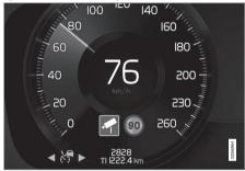
Example of speed camera and speed limit information in the instrument panel
