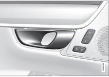
Alternative unlocking method using side door opening handle<sup>11</sup>.
