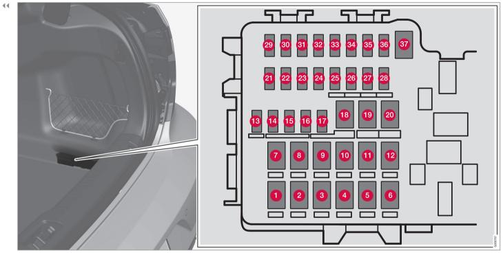
The fuse box is located on the right-hand side.
