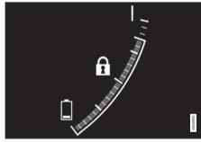
The **A** symbol is displayed in the hybrid battery gauge when Hold is activated.
