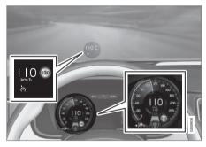
The previous illustration shows that Pilot Assist is set to maintain a speed of 110  $\rm km/h$
