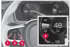
In order to start Cruise Control from standby mode, the vehicle's current speed must be 30 km/h (20 mph) or higher.
