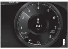
Instrument panel when the paddles are activated for shifting in manual mode.
