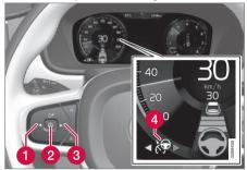
A green steering wheel indicates that Pilot Assist is providing steering assistance.
