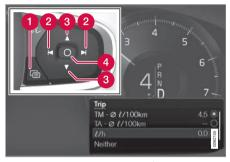
Open and navigate in the app menu<sup>1</sup> using the righthand steering wheel keypad.
