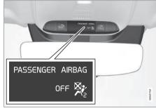
Occupant Weight Sensor (OWS) indicator light
