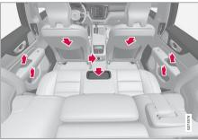
Storage compartment in the door panel, cup holders\* in the center seat's backrest, storage pocket' in the front seat's backrest and USB ports in the tunnel console.
