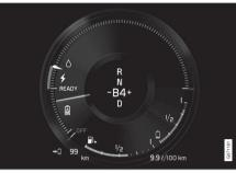
The vehicle is generating current to recharge the battery, e.g. during light braking or engine braking on a downslope.
