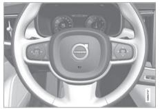
The horn is located in the center of the steering wheel.
