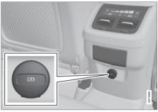
USB ports (type C) on rear of tunnel console for charging phones, tablets, etc.<sup>6</sup>.
