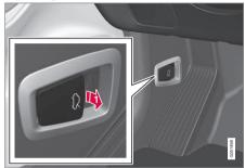
Pull the handle to the left of the brake pedal to release the hood from its fully closed position.
