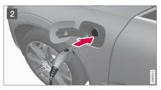
2 Open the charger door. Push the charging handle all the way into the vehicle's socket.
