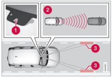
The camera/radar sensor monitors the distance to the vehicle ahead and detects lane markings.
