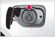
Location of the LED indicator light in the vehicle's charging socket.
