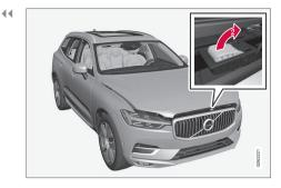
Swipe your hand from left to right under the hood, grasp the handle and move it up and to the side to release the catch and lift the hood.
