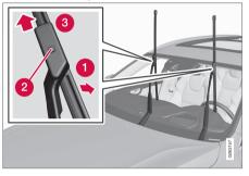
Raise the wiper arms to the service position. Service position is activated/deactivated via the function view in the center display when the car is stationary and the windshield wipers are not on.
