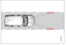
Driver Alert Control detects the vehicle's position in the traffic lane.
