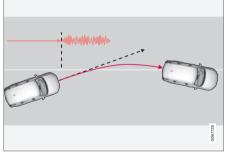
Lane Keeping  $\operatorname{Aid}$  alerts the driver using vibrations in the steering wheel.
