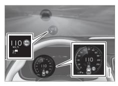
The previous illustration shows that Adaptive Cruise Control is set to maintain a speed of 110 km/h (68 mph) and is following a target vehicle ahead, which is traveling at the same speed.
