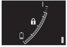
The ft symbol in the hybrid battery gauge indicates that the Hold function is activated. The f symbol indicates that the Charge function is activated.
