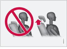
The center head restraint should be adjusted to suit the passenger's height. The entire back of the head should be covered if possible. Manually move the restraint up or down as needed.
