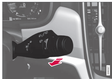
Washing function, right-hand stalk switch.
