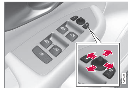
Controls for door mirrors.
