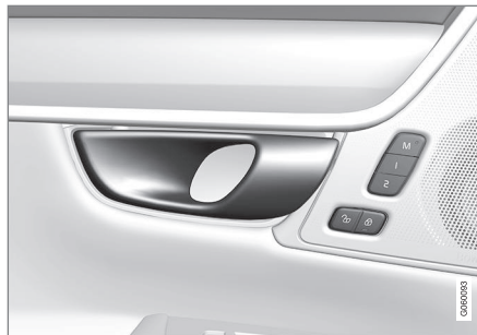
Alternative unlocking method using side door opening handle 11 .
