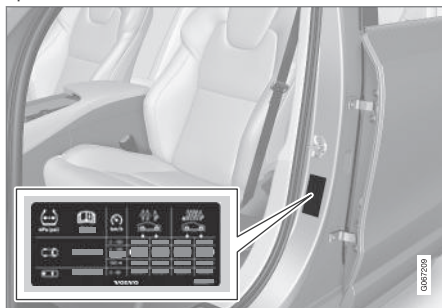
Location of the tire pressure placard
