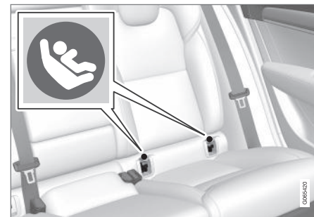
Location of the ISOFIX/LATCH anchors
