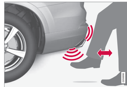
Kicking motion within the sensor's activation area.
