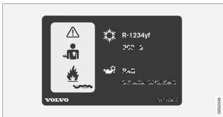
2 Decal for A/C system for cars with refrigerant R1234yf.
