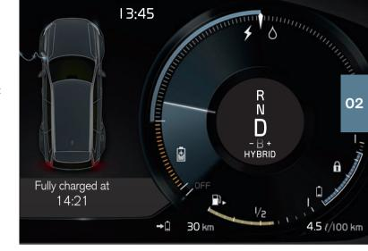
Indicates that the Charge or Hold functions are active. These are activated from the center display's Function view. Charge means that the hybrid battery is being charged if its charge level is low. Hold means that the battery level is being retained for later use.
