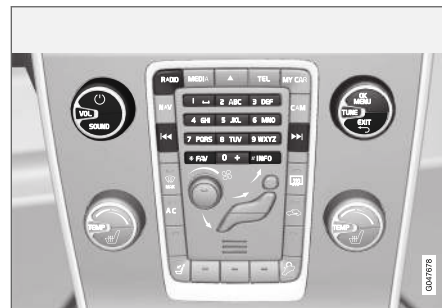
Controls for radio functions.
