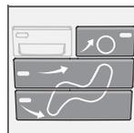
The airflow can be distributed to the windows, dashboard vents or floor by pressing the air distribution buttons.
