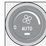
Increase or decrease fan speed by turning the knob. The fan speed is regulated automatically if **AUTO** is selected, and the previously set fan speed is disengaged.
