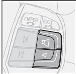
Call volume is regulated with the buttons of the steering wheel keypad.
