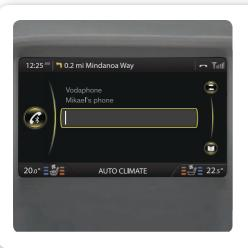
How do I connect a Bluetooth® phone? Press TEL\* in the centre console. 2 Make the external device searchable/visible via Bluetooth<sup>®</sup>. 3 Press **OK/MENU** and follow the instructions on the screen. The device is now connected and can be controlled from the car. In future the phone will be connected to the car automatically.
