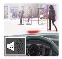
The car has Collision Warning with Auto Brake and Cyclist and Pedestrian Detection, which can warn, brake and/or stop for vehicles, cyclists and pedestrians.
