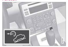
HDC is engaged or disengaged using a switch on the centre console. An indicator lamp in the button illuminates when the function is switched on. When HDC is operating the
