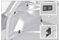
On both sides of the cargo area there are several mounting points designed for securing loads. They are located in the floor and in the top edge of both sides of the cargo area.
