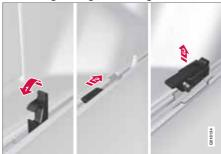
The cargo retaining hooks can be easily removed from the rail, e.g., for cleaning the bottom of the rail.
