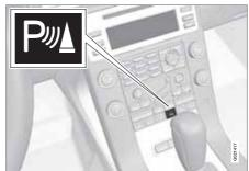
The system is automatically activated when the car is started and the switch's On/Off lamp is illuminated. If parking assistance is switched off with the button, the lamp goes out.
