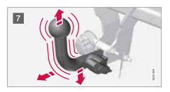
7 Check that the towbar is secure by pulling it up, down and back.
