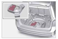
Emergency puncture repair (TMK; Temporary Mobility Kit) is used to seal a puncture and check and adjust tyre pressure. It consists of a compressor and a bottle with sealing fluid. The kit works as a temporary repair. The sealing fluid bottle must be replaced before its expiration date and after use.
