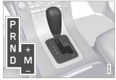
**D**: Automatic gear positions. **M** (+/–): Manual gear positions.
