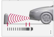
The distance covered in front of the car is about 0.8 metres. The acoustic signal for obstacles in front comes from one of the front loudspeakers.
