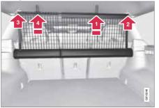
Pull the net up from the cassettes. The net is self-locking after about 1 minute if the rear seat's backrests are raised.
