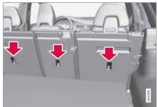
The car is equipped with upper mounting points for certain front-facing child seats. These mounting points are located on the rear of the seat.
