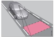
The function is intended to reduce the risk for single-vehicle accidents – accidents where, in certain situations, the vehicle leaves the carriageway and is in danger of driving either into a ditch or into oncoming traffic.
