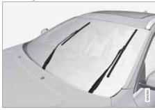
In order to change, clean or lift the wiper blades (for scraping off ice from the windscreen) they must be in service position.
