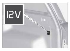
Lower the cover to access the electrical socket. The socket also provides voltage when the remote control key is not in the ignition switch.
