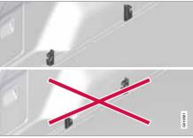
Fit the cargo retaining hooks correctly!
