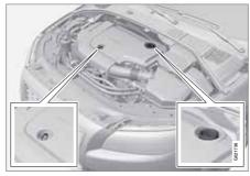
Dipstick<sup>1</sup> and filler pipe, diesel engine.
