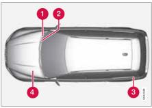
Fuse box locations in a left-hand drive car. In a right-hand drive car the fuse box under the glovebox changes sides.
