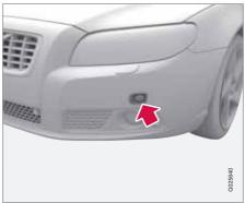
Electrical input to the engine block heater.
