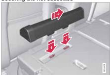
The two-part safety net cassette is secured on the rear of the backrest. The narrowest cassette is secured on the left-hand side (seen from the tailgate).
