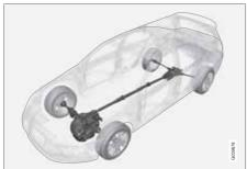
All Wheel Drive means that the car is driving all four wheels at the same time.
