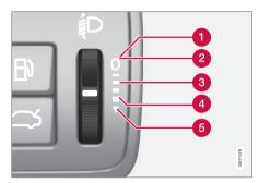
Thumbwheel positions for different load cases.
