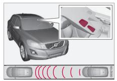
Laser sensor transmitter and receiver window12.
