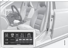
The tyre pressure label on the driver's side door pillar (between frame and rear door) shows which pressures the tyres should have at different loads and speed conditions. This is also specified in the tyre pressure table, see Tyres - approved tyre pressures (p. 422).
