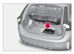
Located under the cargo area floor are the car's towing eye, jack\* and wheel wrench\*. There is also space here for the sleeve for the locking wheel bolts and tools for the plastic wheel bolt caps.
