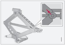
The tools and jack\* must be returned to their correct places after use. The jack needs to be cranked together to the correct position in order to have space.
