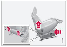
The passenger seat's backrest can be folded forward to make room for long loads.
