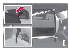
Hook the hook into the load retaining eyelets on both sides and tension the cam lock by pressing down the tongue and tensioning the strap.
