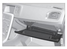
The owner's manual and maps can be kept in here for example. There are also holders for pens on the inside of the lid. The glovebox can be locked\* (p. 183) using the key blade (p. 171).
