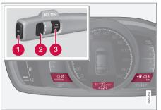
Three trip computer options can be displayed simultaneously - one in each "window".
