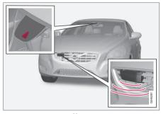
Camera and radar sensor<sup>20</sup>.
