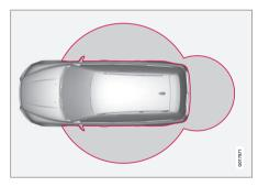
The red rings in the above figure indicate the range covered by the system's antennas.
