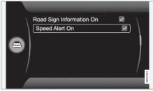
The driver can opt to receive a warning when the applicable speed limit is exceeded by 5 km/h (5 mph) or more. This warning is given by the symbol showing the applicable maximum speed temporarily flashing when this speed is exceeded. The function can be activated/deactivated in the menu system MY CAR. For a description of the menu system, see MY CAR (p. 116).
