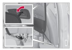
Hook the hook into the eyelet on the seat rail on both sides and tension the cam lock by pressing down the tongue and tensioning the strap.
