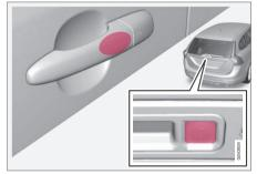
The touch-sensitive area on the outer door handles and the rubberised button next to the tailgate's rubberised pressure plate.
