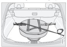
Cars with four load retaining eyelets.
