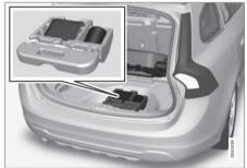
The emergency puncture repair kit is located under the floor in the cargo area.
