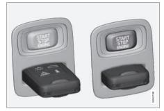
Ignition switch with remote control key extracted/inserted
