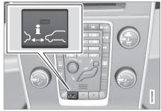
Press the button in the centre console to switch the function on or off. The function is switched on if one lamp is illuminated in the button.
