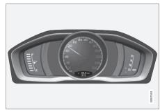
The information from the trip computer can be shown in the combined instrument panel's information display<sup>29</sup>.
