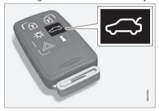
The alarm for the tailgate can be disarmed\* and the tailgate unlocked on its own by using the remote control key's button.
