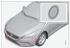
The PAP sensors are located in the bumpers<sup>36</sup> - 6 front and 4 rear.
