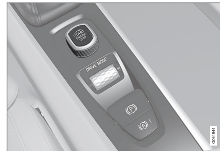
Start knob in the tunnel console.
