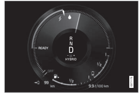
The instrument panel gauge when both the electric motor and the combustion engine are being used.
