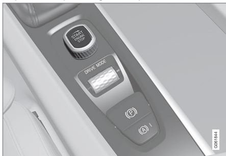
Start knob in the tunnel console.
