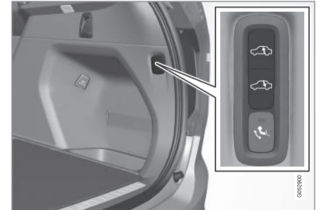
Controls for raising/lowering the car's rear section.
