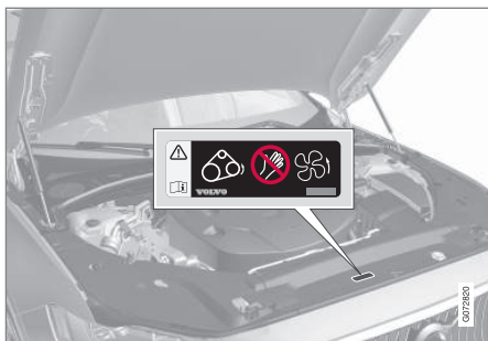
Location of warning decal for the engine compartment. The appearance of the engine compartment may differ depending on model and engine variant.
