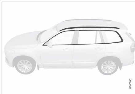
Parts that should be washed using a cleaning agent with a pH value between 3.5 and 11.5.
