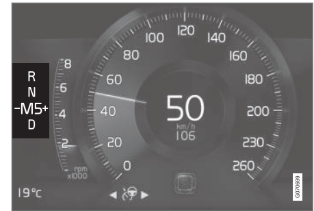
Gear shift indicator in 8-inch driver display for small gear lever.
