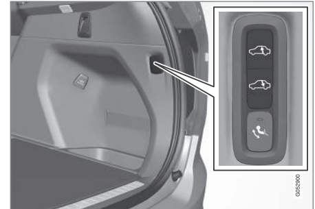
Controls for raising/lowering the car's rear section.
