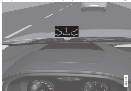
Distance Warning symbol on the windscreen with head-up display.
