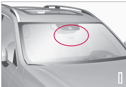
Radar unit location
