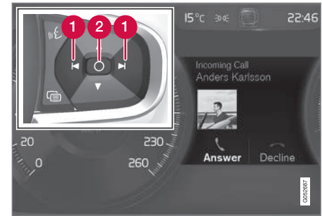
Examples of messages in the driver display 5 and the steering wheel's right-hand keypad. The figure is schematic - parts may vary depending on car model.
