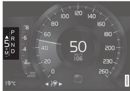
Gear shift indicator in 8-inch driver display for large gear lever.
