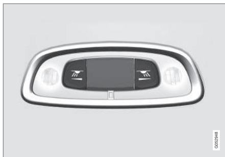
Reading lamps above the rear seat.
