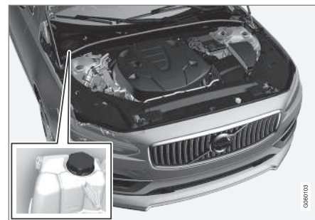
Coolant expansion tank, left-hand drive car
