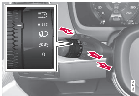
Steering wheel stalk switch with rotating ring.
