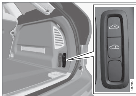
Controls for raising/lowering the car's rear section.
