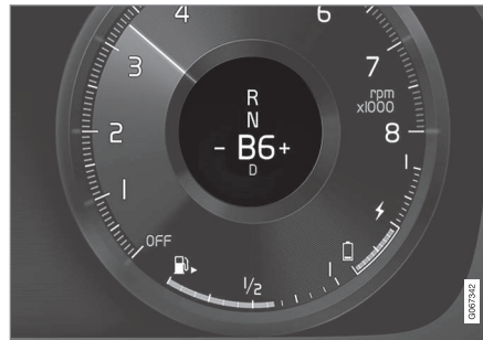
Gear shift indicator in the driver display 5 .
