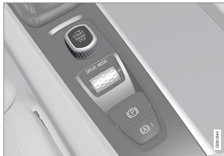
Start knob in the tunnel console.
