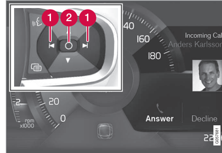
Examples of messages in the driver display 4 and the steering wheel's right-hand keypad.
