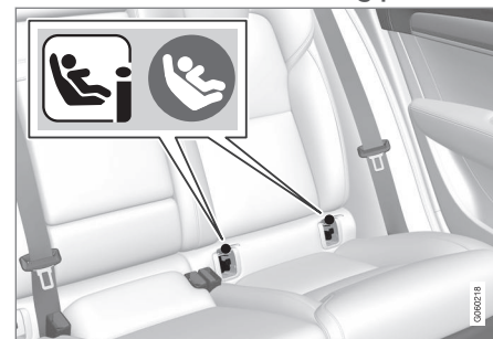
Mounting point locations are indicated by symbols 2 on the upholstery of the backrest.
