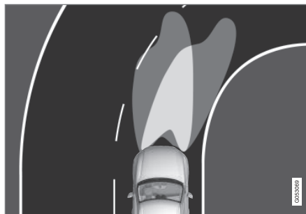
Headlamp pattern with function deactivated (left) and activated (right) respectively.
