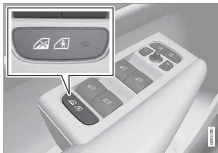
Button for electric activation and deactivation.
