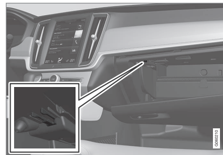
The key's designated storage space. The figure is schematic - the design may vary.
