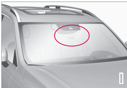
Radar unit location
