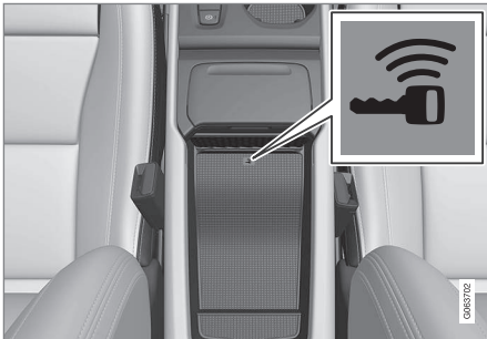
Location of the backup key reader in the storage compartment.
