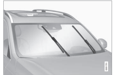
Windshield wipers in the service position.
