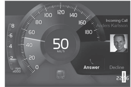
Example of message in an 8-inch instrument panel. The illustration is generic - details may vary according to vehicle model.
