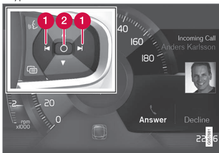
Examples of messages in the instrument panel 3 and the right-side steering wheel keypad.
