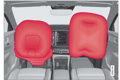
Driver/passenger side front airbags.
