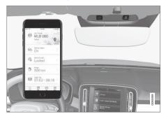
It is possible to lock or unlock the vehicle or check the fuel level directly from a phone or other connected device via the Volvo On Call app. In the event of an accident, emergency assistance (ambulance, police, etc.) can be summoned to the vehicle. In less critical situations, e.g. a flat tire, roadside assistance can be called out.
