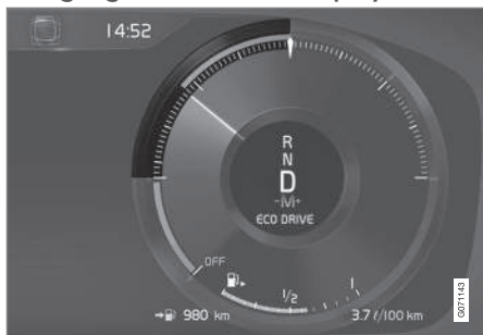
Eco gauge in the 12-inch driver display*.
