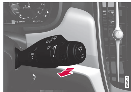
Washing function, right-hand stalk switch.
