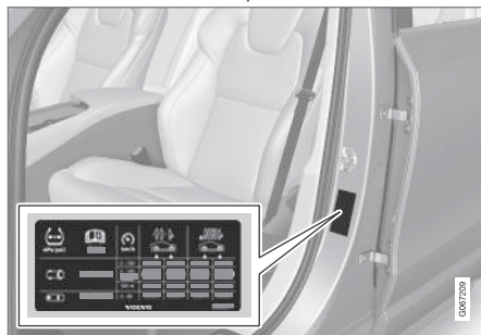
Tyre pressure label location
