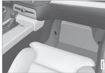
Mounting point locations in the front seat.
