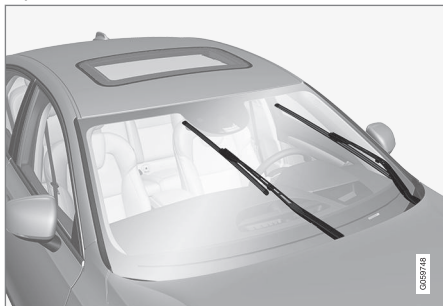
Wiper blades in service position.
