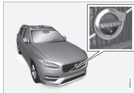
The front Park Assist Camera is located in the grille.
