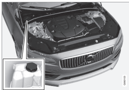
Coolant expansion tank, left-hand drive vehicle
