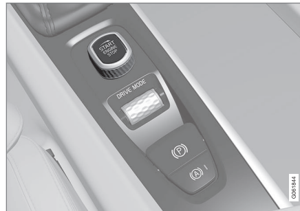
Start knob in the tunnel console.
