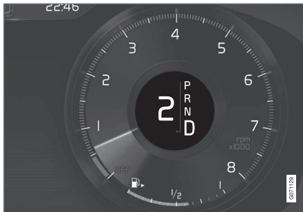
Driver display when changing gear with steering wheel paddles, large gear lever.
