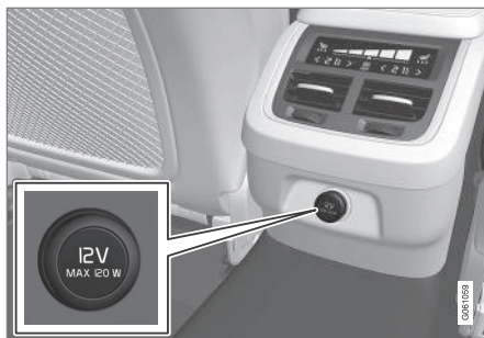
12 V electrical socket in tunnel console, rear seat.
