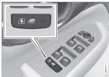
Button for electric activation and deactivation.
