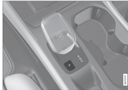
Overview of gear lever and position P.
