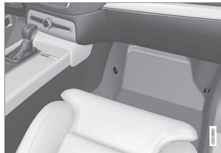
Mounting point locations in the front seat.
