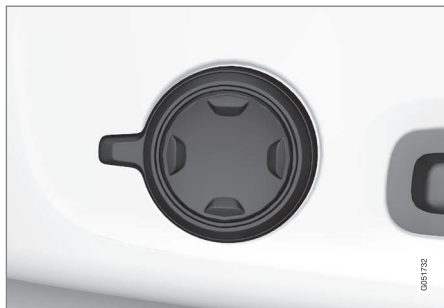
Multifunction control in cars with four-way lumbar support*.
