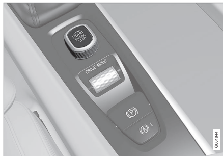
Start knob in the tunnel console.
