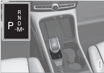
Overview of small gear lever and shift pattern in the driver display.
