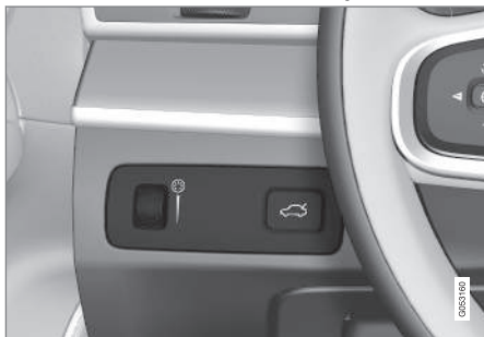
Thumbwheel (to left) for adjusting interior brightness.
