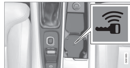
Backup reader's location in the tunnel console.
