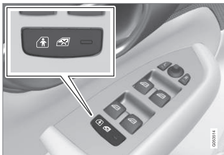
Button for electric activation and deactivation.
