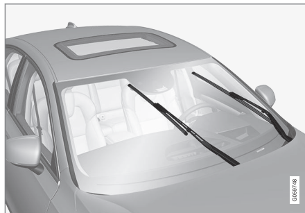
Viskerblade i servicestilling.
