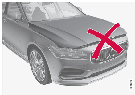
Hood not completely closed.
