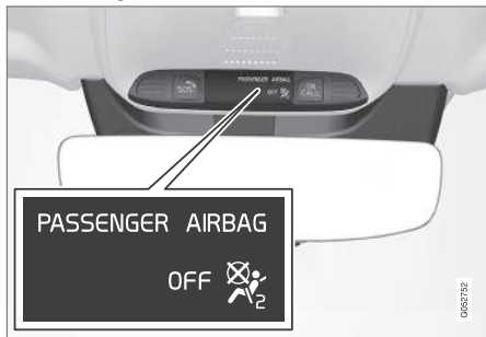
Occupant Weight Sensor (OWS) indicator light
