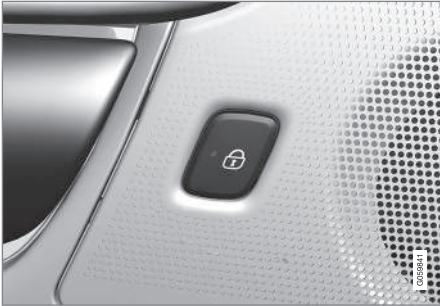
Lock button with indicator light in rear door.
