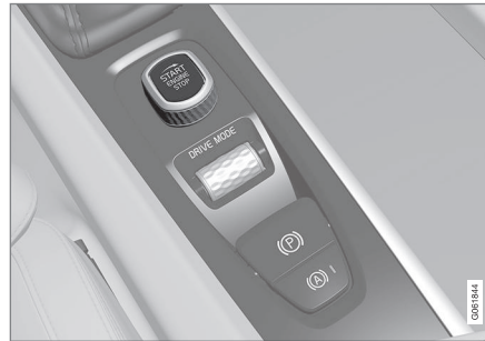
Start knob in the tunnel console.
