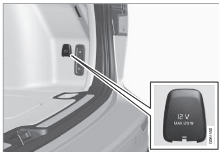
12 V electrical socket in cargo area*.
