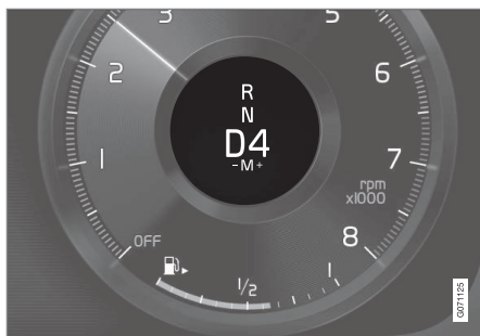
Driver display when changing gear with steering wheel paddles, small gear lever.
