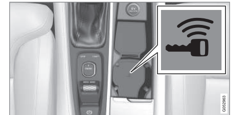
Backup reader's location in the tunnel console.
