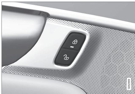
Lock buttons with indicator lamp in the front door.
