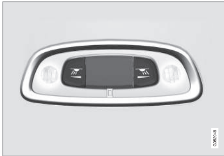
Reading lamps above the second 17 and third seat row*.
