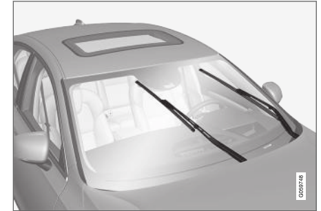
Viskerblade i servicestilling.
