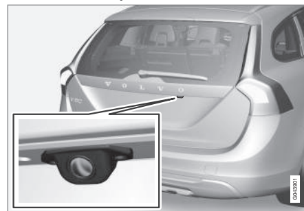
Camera location next to the opening handle.
