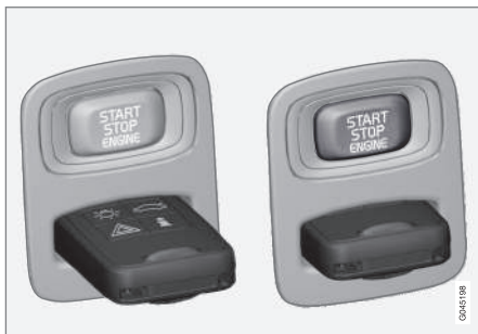
Ignition switch with remote control key extracted/inserted.
