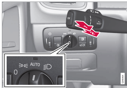
Stalk switch and knob for headlamp control.
