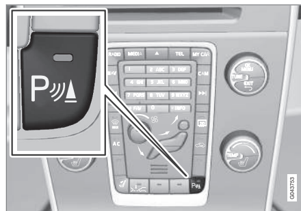
On/Off for parking assistance and CTA sensors.
