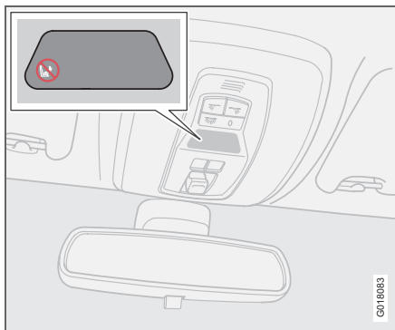
Indicator showing that the passenger airbag (SRS) is activated.
