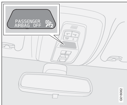
Indicator showing that the passenger airbag (SRS) is deactivated.
