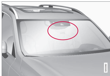
Radar unit location.
