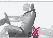
Do not leave any objects on the floor behind the driver's seat/passenger seat that may prevent the WHIPS system from functioning.
