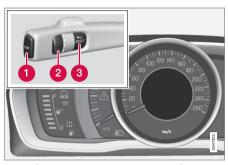
Display (analogue combined instrument panel) and controls for menu navigation.
