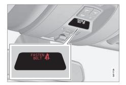
The audio reminder is speed dependent, and in some cases time dependent. The visual reminder is located in the roof console and in the combined instrument panel (p. 66).
