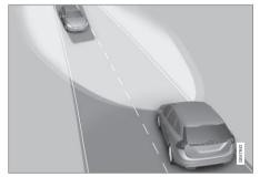
Adaptive functionality: Dipped beam directly toward oncoming vehicles, but continued main beam on both sides of the vehicle.
