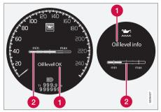
Message and graphic in the display. The left-hand display is shown in the digital combined instrument panel and the right-hand in the analogue.
