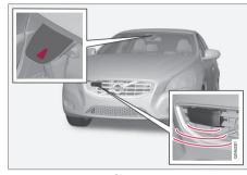
Camera and radar sensor<sup>21</sup>.
