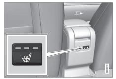
Current heat level is shown in the pushbutton's lamps.
