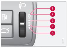
Thumbwheel positions for different load cases.
