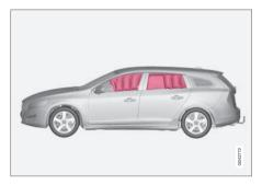
Inflatable curtain IC (Inflatable Curtain) is part of the SIPS system (p. 38) and the airbag system (p. 33). It is fitted along both sides of the headlining and helps protect the driver and passengers in the car's outer seats. A sufficiently violent collision trips the sensors and the inflatable curtain is inflated.
