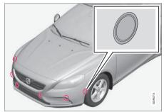
The PAP sensors are located in the bumpers<sup>37</sup> - 6 front and 4 rear.
