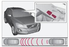
Laser sensor transmitter and receiver window<sup>13</sup>.
