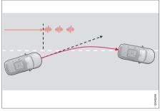
Warning with steering wheel vibration<sup>27</sup>.
