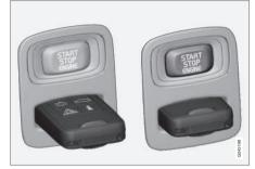
Ignition switch with remote control key extracted/ inserted.
