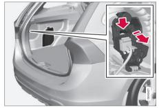
The bulbs for reversing lamp, fog lamp and direction indicator in the rear lamp cluster are replaced from inside the cargo area.
