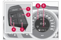
The steering wheel buttons and combined instrument panel in cars **without** speed limiter<sup>2</sup>.
