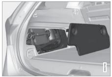
The towing hitch is stowed together with the tools behind a side hatch in the cargo area.
