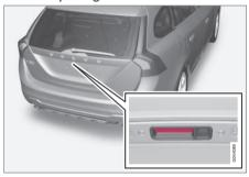
Rubber plate with electrical contact.
