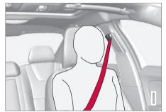
Correctly fitted seatbelt.
