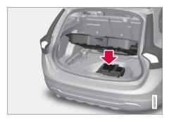
Located under the cargo area floor are the car's towing eve, jack\* and wheel wrench\*. There is also space here for the sleeve for the locking wheel bolts and tools for the plastic wheel bolt caps.
