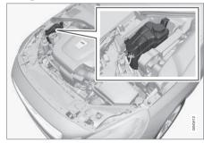
When topping up the coolant, follow the instructions on the packaging. Never top up with water only. The risk of freezing increases with both too little and too much coolant concentrate.
