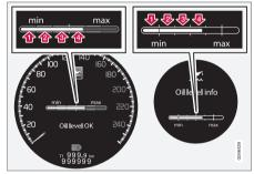
The figures 1-4 represent filling level. Do not fill more oil if filling level (3) or (4) is shown. Recommended filling level is 4.
